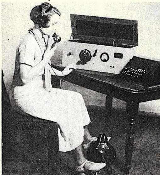
With power from pedaled generators, radio sets are used to summon or receive medical aid. Up to 200 miles, radiophone conversation is used. Over 200 miles, Morse code dots and dashes are sent out by an automatic keyboard when proper key is pressed. This device eliminates necessity for knowing codes.
