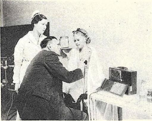
Through the use of this electrical stethoscope, developed by Western Electric Company, physicians can hear heart murmurs formerly impossible to detect with ordinary stethoscope.
