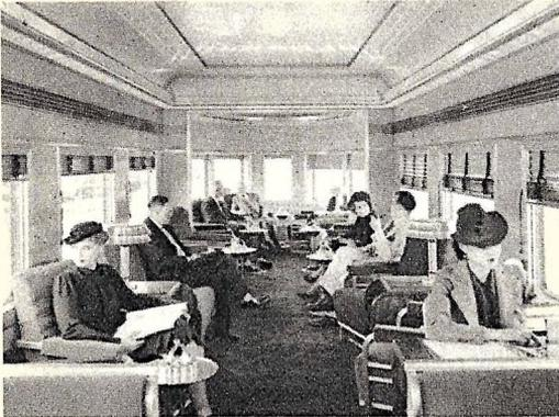
The new Pullman observation cars are roomy and comfortable. Steel alloy bodies and aluminum alloy interiors, comfortable seats, venetian blinds, and indirect lighting are featured.
