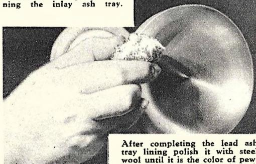
After completing the lead ash tray lining, polish it with steel wool until it is the color of pewter. Lock lining in wood bowl.
