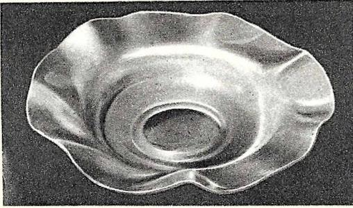
This attractive dish makes a novel pin tray when completed. After successfully completing the aluminum coaster you are ready to advance to this project which is spun from aluminum.
